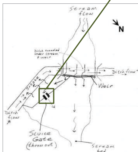
Ratchet sluice gate throw-out at Kaaiea stream diversion. View facing S
